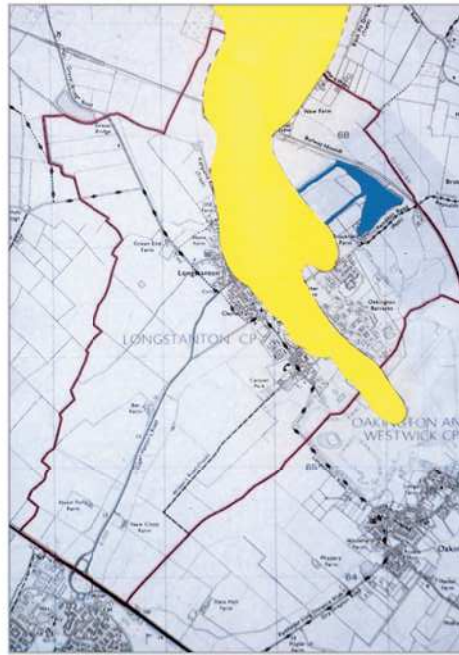
Map of Longstanton Parish boundary (red) illustrates the approximate location this gravel bed, (yellow) and importantly the large ditches (blue) that have been cut, apparently, to drain water from the gravel bed to the balancing ponds.
